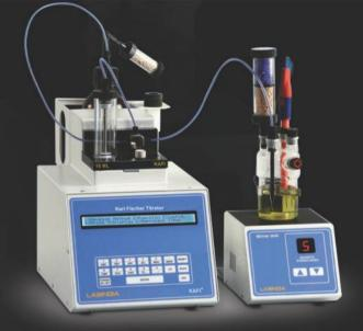
Karl Fischer titration is an accurate, rapid and efficient method for determining the water content in samples. When the sample is titrated in the presence of  $SO_2$ ,  $I_2$ , and an organic base, moisture from the sample extracted in the solvent, can be quantitatively estimated. Dry methanol is used as a solvent in Karl Fischer titration.
